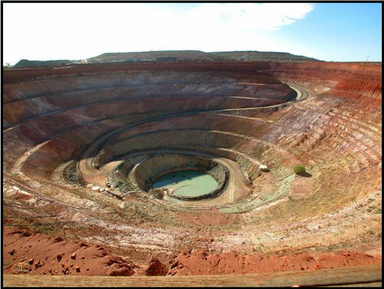
Figure 2: An example of the open-pit method
