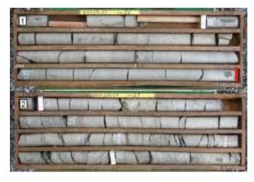
Figure 2: Typical examples of a Drilling rig and Core Logs.
